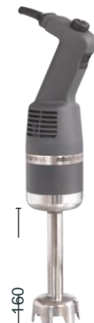
PML0160 POWER MIXER MINI - MP 160 V.V. (KNIFE AND EMULSIFYING DISC INCLUDED) SPECIFICATIONS LENGTH OF TUBE: 160mm - Ø78mm TOTAL LENGTH: 430mm VARIABLE SPEED: From 2000 to 12500rpm MOTOR POWER: 220W - Single phase 230V - 50Hz
