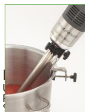
PMC0300 POWER MIXER COMPACT - 300 V.V. - 30Lt (KNIFE INCLUDED) SPECIFICATIONS LENGTH OF TUBE: 300mm - Ø94mm TOTAL LENGTH: 660mm VARIABLE SPEED: From 2300 to 9600rpm MOTOR POWER: 350W - Single phase 230V - 50Hz
