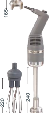
PMM0165 POWER MIXER MICROMIX (KNIFE AND EMULSIFYING DISC INCLUDED) SPECIFICATIONS LENGTH OF TUBE: 165mm - Ø78mm TOTAL LENGTH: 470mm VARIABLE SPEED: From 2000 to 14000rpm MOTOR POWER: 220W - Single phase 230V - 50Hz
