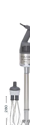
PML1450 POWER MIXER LARGE - MP 450 COMBI ULTRA (WHISK AND KNIFE INCLUDED) SPECIFICATIONS LENGTH OF TUBE: 450mm - Ø125mm TOTAL LENGTH: 890mm WITH WHISK: 840mm VARIABLE SPEED: From 1500 to 9000rpm (Mixer function) From 250 to 1500rpm (Whisk function) MOTOR POWER: 500W - Single phase 230V - 50Hz
